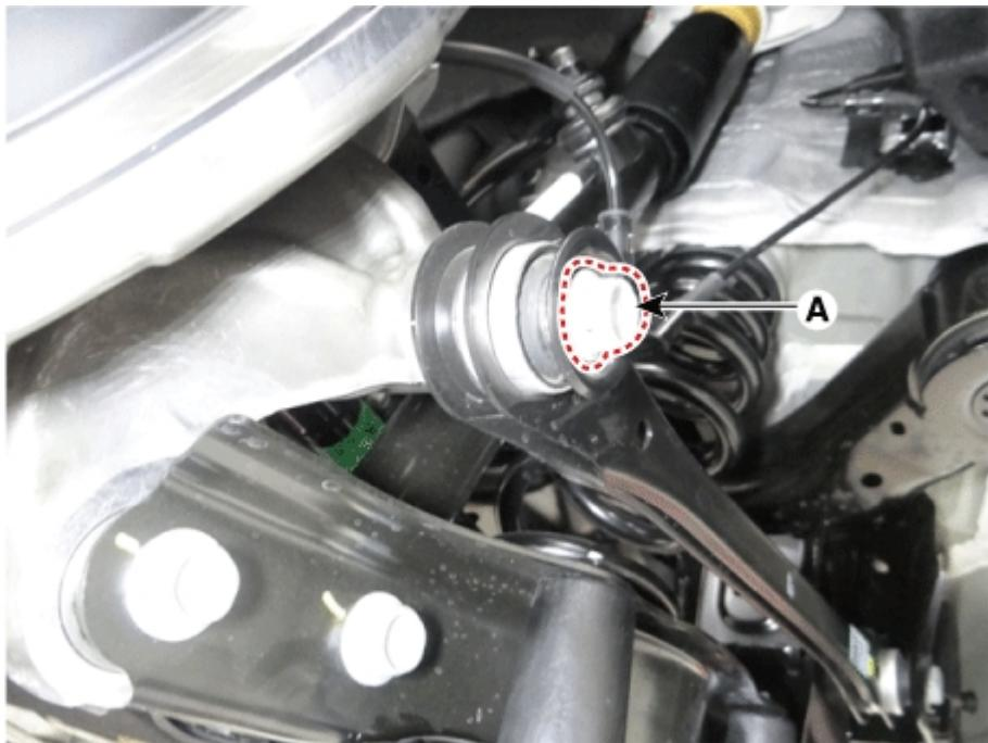
10. Loosen the bolt & nut and then remove the rear upper arm front from the rear axle.
