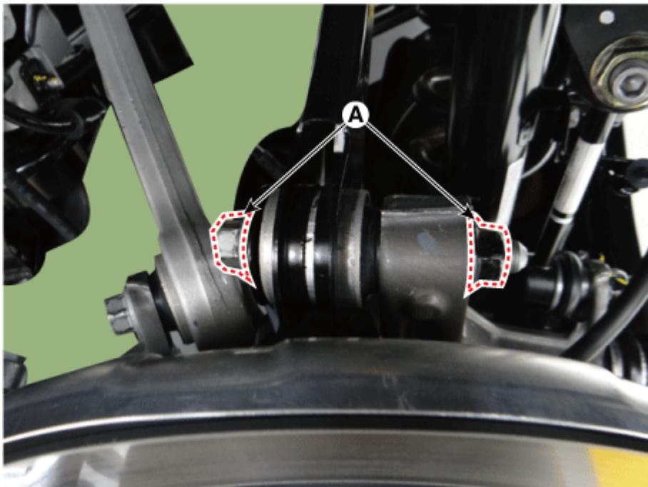
12. Separate the rear drive shaft from the knuckle.
