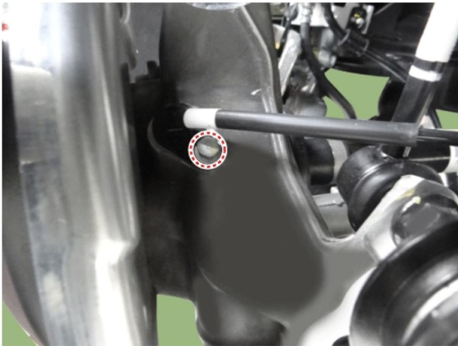
6. Loosen the stabilizer link nut and then separate the rear axle.
